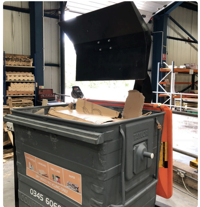
CC1100 — COMPACTING HEAD LOWERED (LEFT) AND RAISED FOR LOADING (RIGHT)
